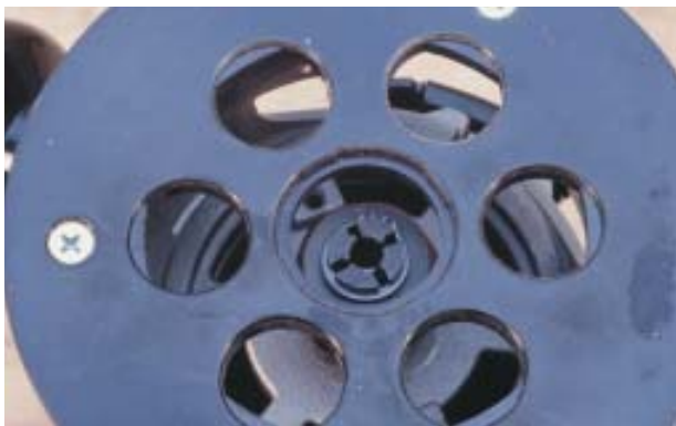
To use Porter-Cable-style bushings, you need a sub-base with a small center hole.
