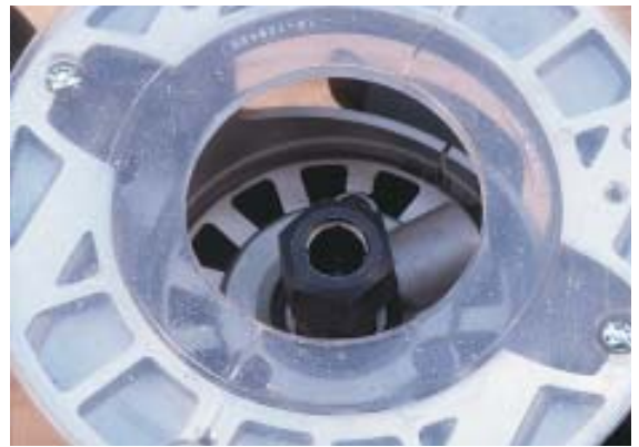
For large-diameter bits, you need a sub-base with a big center hole. DeWalt uses clear plastic sub-bases to make it easier to see the work.
