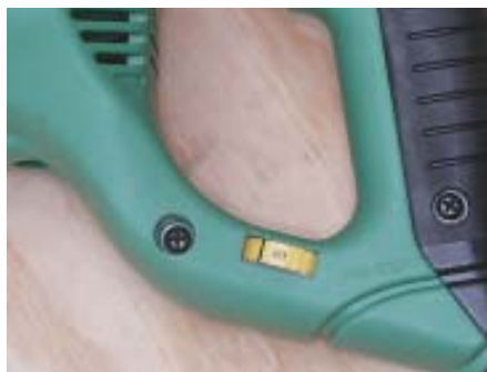
The Hitachi CR13VA is one of a few saws with an auxiliary speed dial that allows you to set an upper limit on the speed of the blade. It comes in handy for long low-speed cuts.
