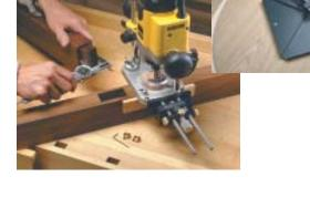
**A Cut Above.** Some cuts you simply can't afford to mess up; stair treads are among them. But you can practically guarantee accurate cuts and a tight fit with the *Stairtool*, a well-made aluminum template with the single purpose of fitting treads on a finished stair-
