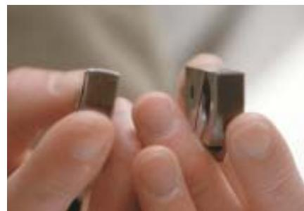
**With flat- and rounded-sole models, the Bunny Plane can clean up scarf joints on most molding. Five different rounded blades add to the versatility.**
