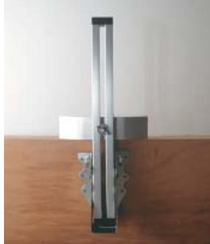
Adjustable for joist hangers up to 12 inches, the JoistMate keeps the hanger straight and frees one of your hands for starting nails. Using the red alignment mark behind the wingnut speeds joist layout, because you need to make only one layout mark.
