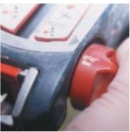
A front-mounted lever, located to the left of the miter control, allows the user to adjust bevel settings without reaching behind the saw. Although the saw can bevel up to 47 degrees, stops prevent going past 45 degrees for ordinary tasks (left). An override knob, located on the other side of the miter control, deactivates the stop for taking bevels past 45 degrees (right).
