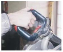
The four-position handle improves comfort and control for making difficult cuts. Unlocking a metal draw-catch frees the handle for adjustment. Although the handle seems sturdy, the manufacturer includes a secondary handle for transport.
