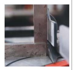
A try square highlights the discrepancy between the fence and the extension wing mounted on top. A steel shim between the fence and the extension wing helped, but the alignment was still off.
