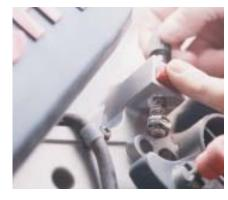
The depth stop on the 4412 adjusts quickly. A button disengages the threads for rough adjustments; releasing the button and turning allow fine-tuning. A sturdy, low-tech jam nut holds the proper setting.
