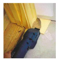
This miter table excels at cutting shoe mold and quarter round — small profiles that can be downright exciting to cut in my 12-inch miter saw. While building a fireplace mantle, I clamped the miter table to a sawhorse set up nearby and was impressed by the speed and time saved by cutting small pieces right at hand. I found the table's accuracy to be just fine.
