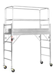
and has a 500-pound load rating. It's adjustable in 2inch increments from 3 to 6 feet tall. Best of all, the entire platform (without toe boards or rails) weighs only 80 pounds. It sells for \$345. Lynn Ladder, 800/225-
