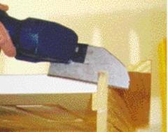
Faster than a handsaw and more precise than a circular saw, Bosch's 1640 reciprocating blade makes quick work of trimming doorjambs. The blade is reversible for flush cutting on either side of the jamb.
