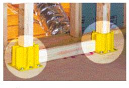
**Rail Supports.** Temporary safety rails don't have to be a huge production. The Safety Boot is an easy-to-use temporary safety rail system meant to protect workers from falling down stair openings or off balconies. The plastic boots receive ordinary construction-grade 2x4s, and they can be screwed directly to the floor surface. According to the manufacturer, the Boots' high-impact polymer will last for years. They retail for about \$23 each.
