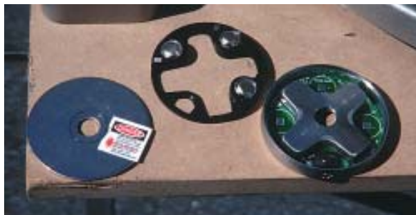
Three watch batteries power the laser.
