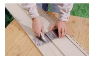
The *Sider*'s  $^{1}$ /8-inch graduated slots receive a utility knife and make quick work of long parallel cuts. The aluminum template is available to match most vinyl siding profiles, including double 4 and 5, dutch lap  $4^{1}$ /2 and 5, and triple 3. The stainless-steel marking gauge sells for about \$16.
