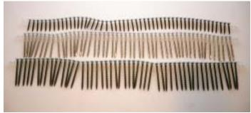
Screws load from the top of the DS300, which keeps them from poking you in the leg while you're using the tool. The 50-screw collations feed consistently, and the screws seem to be of high quality, with sharp points.
