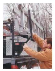
your Tapco or Van Mark metal brake to your truck's ladder rack, which not only saves space in the bed of your truck, but also creates a convenient work station. According to the manufacturer, the Brake Rack makes your expensive metal brake harder to steal, as well. It sells for about \$230.
