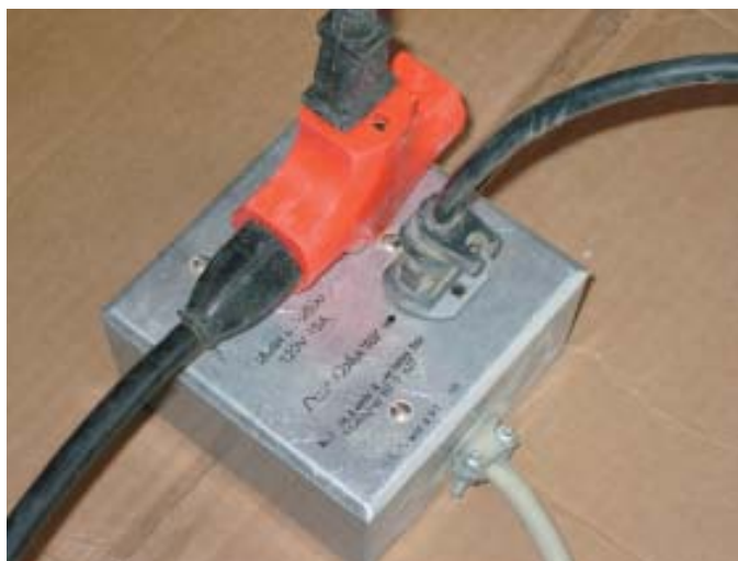
Figure 5. The vacuum is activated by an automatic switch that senses when a saw comes on. A number of dust-collecting vacs are available with a similar feature.
