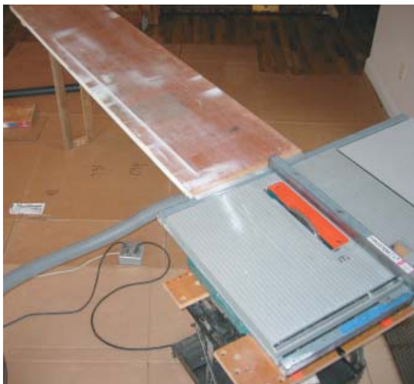
Figure 7. If the table saw is used alone it can be outfitted with a wider outfeed table (left). The outfeed connects to the saw with a piece of angle and is held in place by a pin (above).
