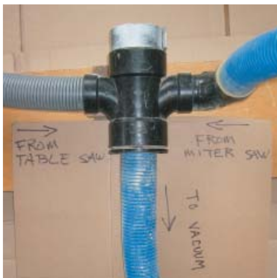
Figure 6. A homemade air valve is made from standard plumbing and electrical fittings (above). Rotating a piece of plastic conduit directs suction to a particular saw. At right, the author has pulled the conduit out to reveal the hole that directs the air.
