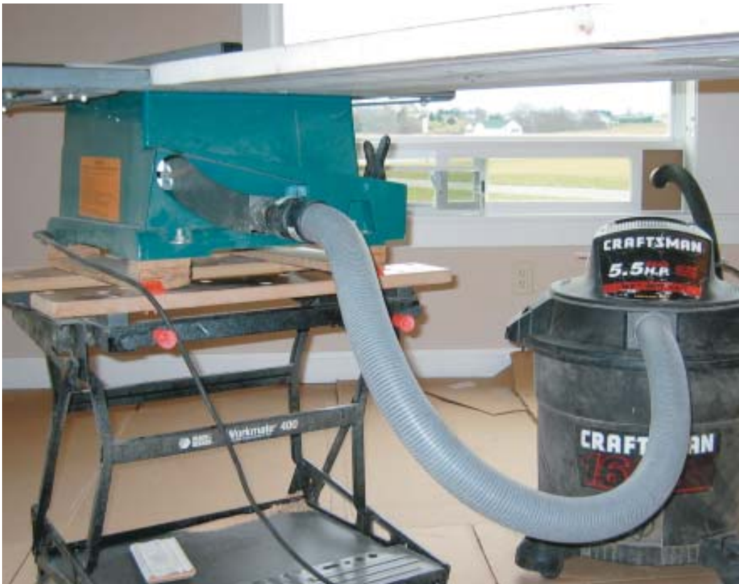
Figure 3. Blocks bolted to the bottom of the saws are grasped between the dogs on top of the WorkMates. In this setup, the saw is connected directly to the vac, which exhausts the dust out the window.
