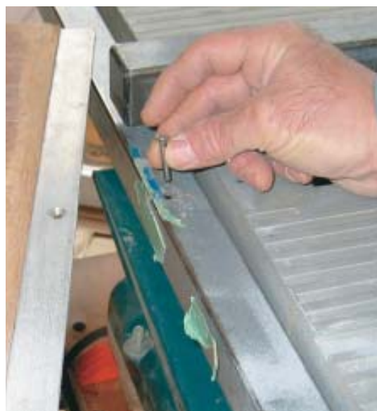
Figure 7. If the table saw is used alone it can be outfitted with a wider outfeed table (left). The outfeed connects to the saw with a piece of angle and is held in place by a pin (above).
