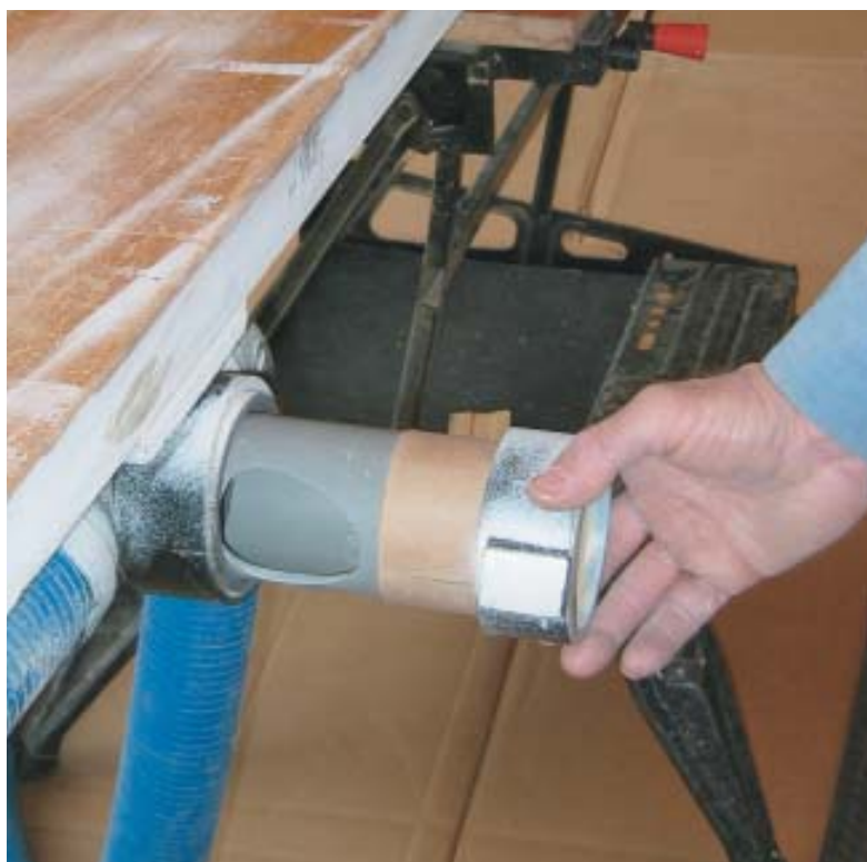
Figure 6. A homemade air valve is made from standard plumbing and electrical fittings (above). Rotating a piece of plastic conduit directs suction to a particular saw. At right, the author has pulled the conduit out to reveal the hole that directs the air.
