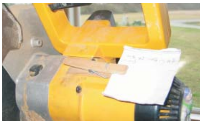
Figure 8. It's easier to keep track of what you're doing if your cut list is where you can see it and won't get lost. The author achieves this by gluing a clothespin to the housing of his saw.
