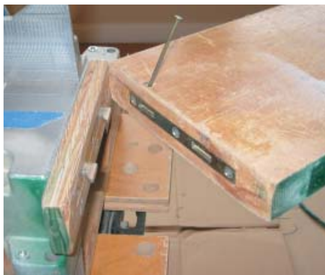
Figure 2. The wings are tied to the saw by bed rail connectors. The author prevents them from accidentally popping free by jamming the hardware with a nail.
