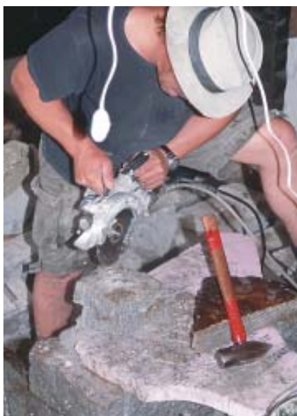
Figure 7. The author's saws are modified with a pump-fed water tube to lubricate the stone during cutting. Dry-cutting is also possible but drastically shortens blade life.
