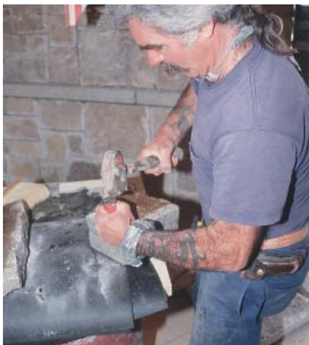
Figure 8. “Rocking” the cut edges with a chisel or masonry hammer gives the stone a more natural look.
