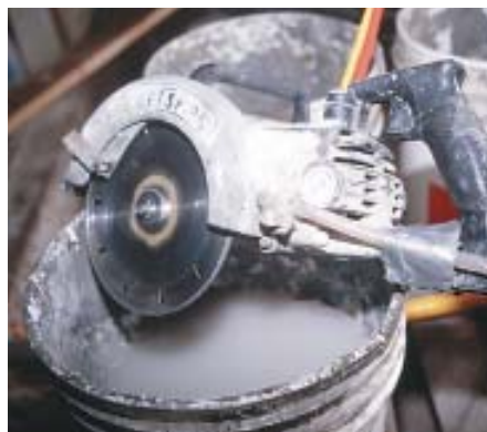
Figure 7. The author's saws are modified with a pump-fed water tube to lubricate the stone during cutting. Dry-cutting is also possible but drastically shortens blade life.
