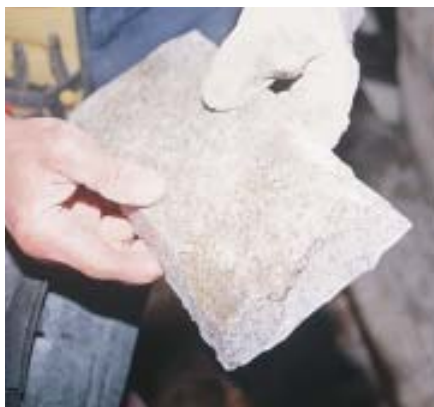
Figure 2. An ashlar pattern requires each stone to have straight, man-made edges and be laid in a close-fitting, angular design. The waste factor runs as high as 40%, producing a considerable pile of rubble as the work progresses.
