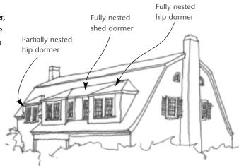
The separate partially nested hip dormer is formed by extending the exterior wall plane up through an interrupted eaves line. This dormer's placement, roof, and window configuration reflect the neighboring fully nested dormers, helping it to fit in and to tie together the overall elevation.
