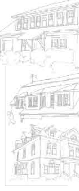
house may appear overwhelming and no longer secondary to the primary roof. In the other extreme, dormers that are too small may appear lost within the roofscape, and more of a blemish than a benefit. Use dormer placement and scale to enhance and clarify building function and massing.
