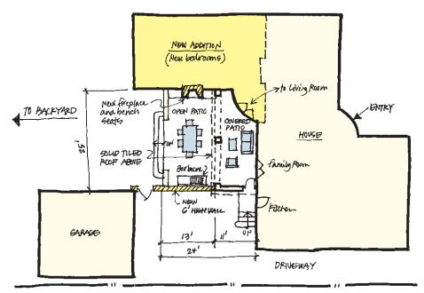
The addition of a new bedroom wing to this two-story Mediterranean created a sheltered angle that was ideal for an outdoor living space. The roofed portion nearest the house provides a refuge from the afternoon sun. A new wall separates the driveway from the living area, but a gate provides easy access between the two.
