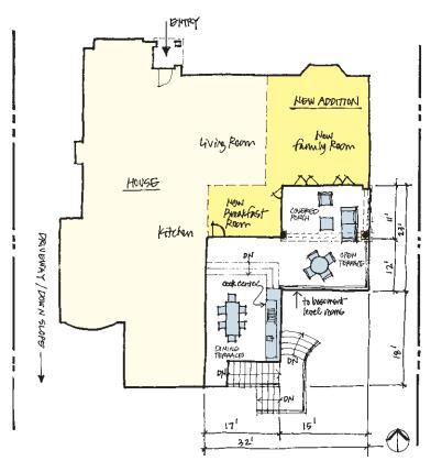
On this steep site, the floor of the upper terrace and porch also serves as the roof of the new basement-level family room–game room below. The floor system consists of I-joists covered with plywood, a waterproof membrane, and brick in thinset cement. The curved lower stairs lead to the family room, while the straight stairs lead to the backyard and driveway.
