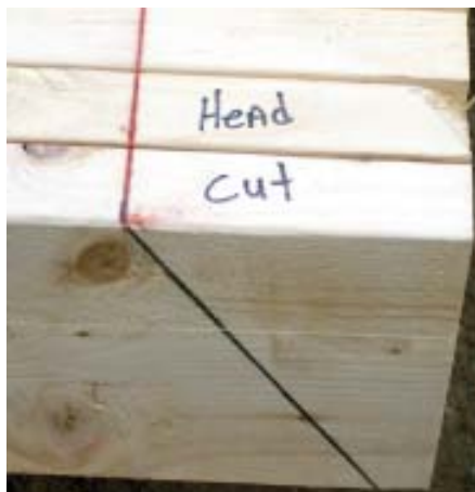
Figure 2. Layout is done on the outer pieces (right), and a chalk line is used to transfer the cut lines to the pieces in between (below).
