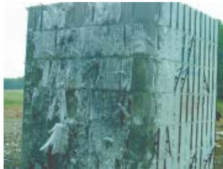
A poured concrete box, protected by foam forms, shows no structural damage from a 50-pound TNT charge detonated 6 feet away.
