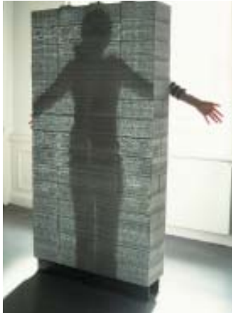
Glass fibers in the mix let LiTraCon concrete blocks achieve translucency, opening up a new set of options for daylighting and nighttime illumination in concrete construction.
