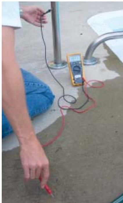
Homeowner Lonn Rickstrom measures 2 to 4 volts to ground at poolside (left) and at his gas meter (right). Wet skin allows current to flow through people, causing a tingling sensation, at voltages below this threshold.
