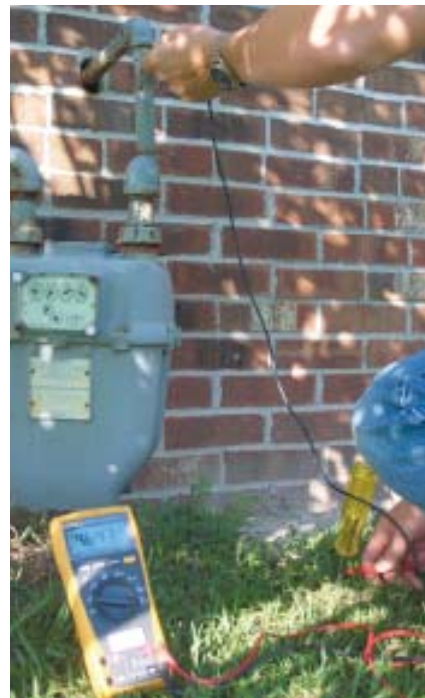
Homeowner Lonn Rickstrom measures 2 to 4 volts to ground at poolside (left) and at his gas meter (right). Wet skin allows current to flow through people, causing a tingling sensation, at voltages below this threshold.
