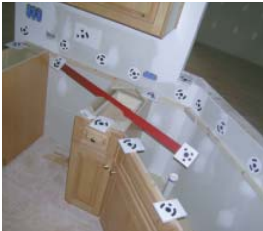
Figure 4. Proprietary plastic "Intelli-Mark" markers center target dots on cabinet edges. User-defined graphic codes inform the software of each marker's significance in the pattern.
