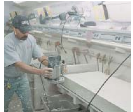
Figure 2. Task-specific tools are within easy reach on the above-bench racks (above). The topless, flip-up bench arms can be configured to suit various jobs. Vacuum ports above the bench provide efficient dust control (left), while blowers below the bench warm the material for rapid glue-ups. The table saw folds down out of the way when not in use (below).
