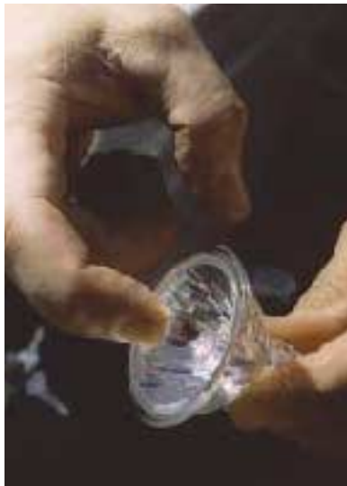
Figure 9. Landscape lighting circuits and fixtures are constantly exposed to weather and have to be able to withstand moisture. To protect wire splices, the author uses a two-piece fitting from Blazing Products (left) that uses an O-ring and a silicone-filled cap to seal out moisture. The author chooses MR (“metallic reflector”) lamps equipped with glass shields that protect the lamp from any drips of condensation that may form inside the weather-sealed lighting fixture. At right, he taps on a lamp’s glass protector shield.
