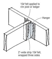
corrosion, I isolated all metal framing connectors from the treated framing with pieces of 15# felt. Each joist hanger needed two pieces, one applied to the ledger board or rim joist, and one strip a few inches wide wrapped around the three sides of the joist resting in the hanger.
