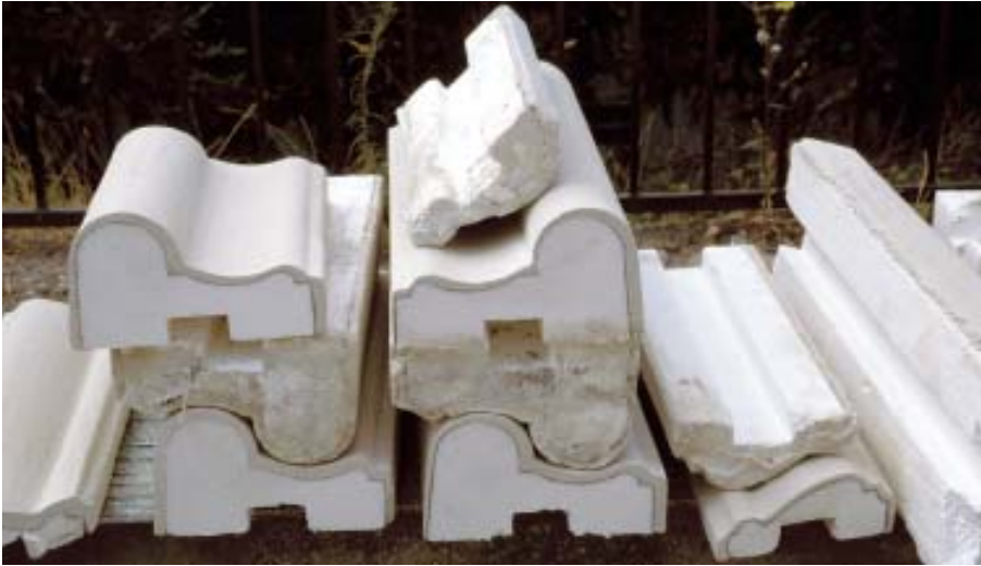
Figure 3. The author creates faux limestone in his shop by applying a polymer-concrete coating to foam profiles (left). His crew cuts the trim in the field, glues it to the building, and mortars the joints. When complete, it's hard to distinguish from real stone (below).
