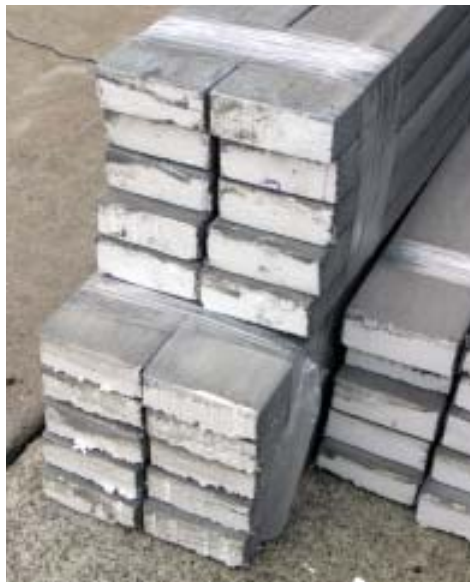
Figure 2. On this job, raw foam has been glued to the wall (left). It will be covered with fiberglass mesh and given a faux stone finish. It's faster to use precast foam; the material shown in the photo at right arrived on site with the mesh and a cementitious coating already on it.
