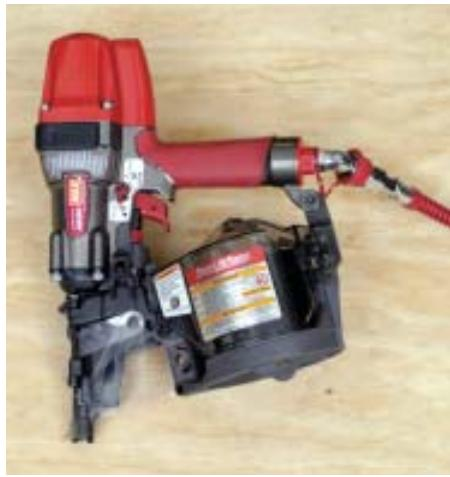
Even fully loaded, this coil framing nailer weighs less than stick nailers
