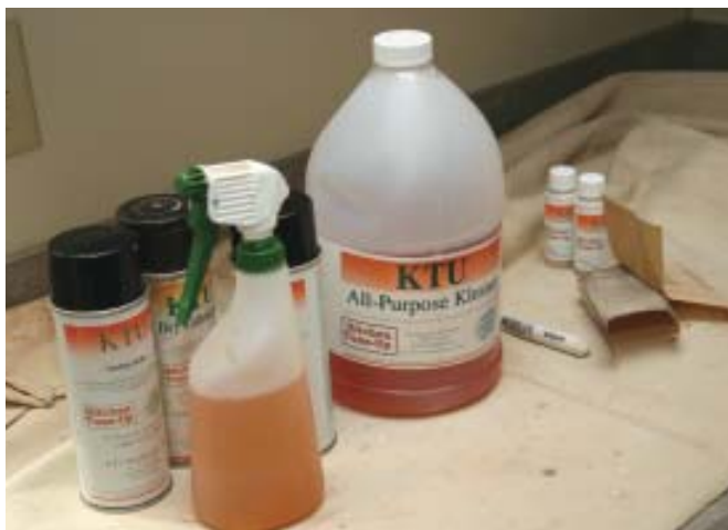
Figure 3. Wax stripper, wood cleaner, and scratch-filler products prepare worn cabinets for a renewed finish of penetrating oils and color lacquer.
