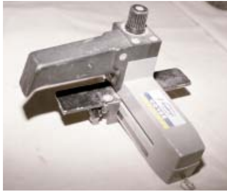
Figure 7. The authors purchase wood veneer in sheets backed with PSA (pressure-sensitive adhesive) and slice it on the job as needed. A hand-held laminate splitter speeds this work.
