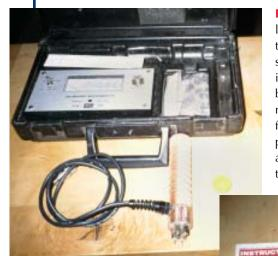
Pin-type moisture meters (left) leave holes in the wood, while the slightly more costly nondestructive type (below) can read interior moisture <sup>3</sup>/<sub>4</sub> inch beneath the surface without marking the piece. Readings from either should be interpreted for different wood species according to charts supplied by the instrument suppliers.
