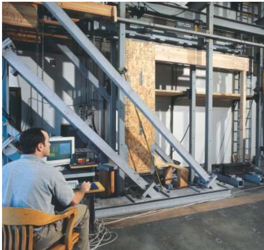
Figure 1. APA determined the nailing schedule for the Narrow Wall Bracing Method by building the assembly and testing it under measured loads.
