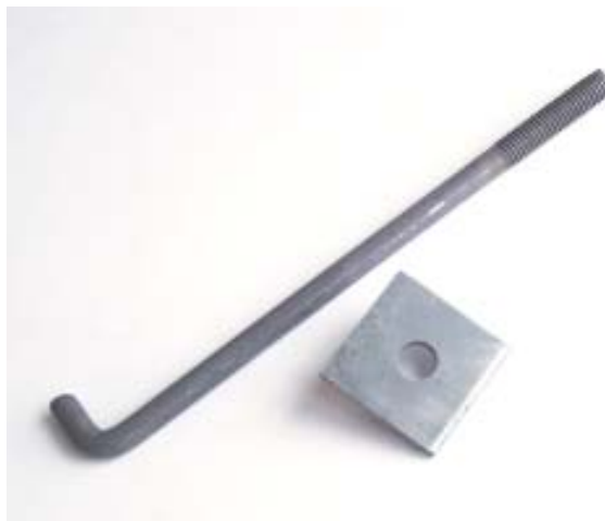
Figure 3. Standard anchor bolts and \frac{3}{16} -inch-thick square washers available from metal connector manufacturers secure the narrow wall to the foundation stem wall.
