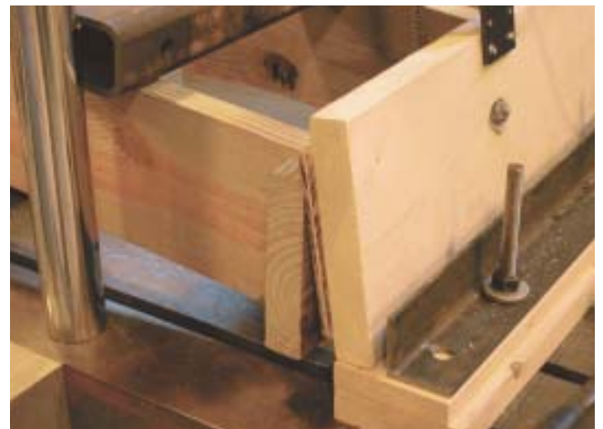
Figure 2. The hydraulic test machine put pressure on a pair of joists attached by hangers to the sample ledger (above). Extra fasteners in the hangers ensured that failure would occur not at the hanger but in the lag screw or bolt attaching the sample ledger to the sample band joist. A transducer measured displacement of the ledger (above right), while a computer continuously recorded measurement and load data. The load was applied until the connection failed (right).
