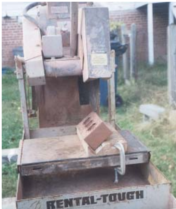
Figure 2. A wood jig clamped to the sliding table of the saw holds the brick at a 45-degree angle for safe cutting.
