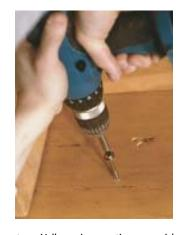
**Sturdy Screws.** Not that long ago, attaching structural components required bolts or lag screws, but several years ago GRK introduced *Self-Drilling Structural Screws*. These sturdy and innovative fasteners provide two to three times the shear strength of comparably sized lags, making them perfect for ledgers to landings. They're available in lengths from approximately 2 to 16 inches in <sup>1</sup>/4-, <sup>5</sup>/16-, and <sup>3</sup>/8-inch diame-
