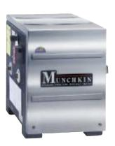
ratings as high as 199,000 Btus. It weighs about 100 pounds and has an extremely small — 31x21-inch — footprint, so it can fit in places where other boilers won't go. But that's not all that's noteworthy: The computer-controlled Munchkin has a stainless-steel heat exchanger and a 92% efficiency rating, and you can vent it through the roof or sidewall with 3-inch ABS, PVC, or CPVC pipe.
