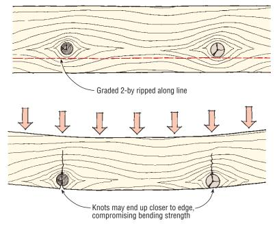
Ripping a piece of graded lumber to make a narrower beam is disallowed by code because it may place strength-reducing characteristics like knots close to the edge of the board, compromising bending strength.
