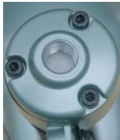
Figure 5. A built-in filter protects the innards of the gun by preventing the entry of dirt and grit.
