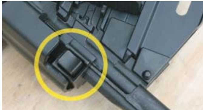
Figure 2. A push-button release allows you to extend and retract the contact element on this Bostitch gun.
