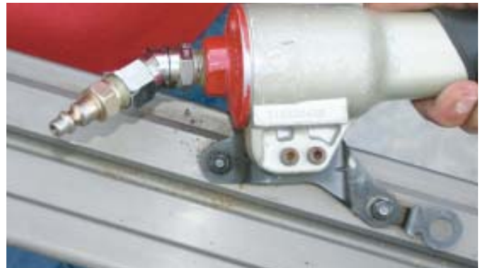
Figure 4. A useful "extra," the swivel fitting on the Max nailer helps prevent hose kinks.
