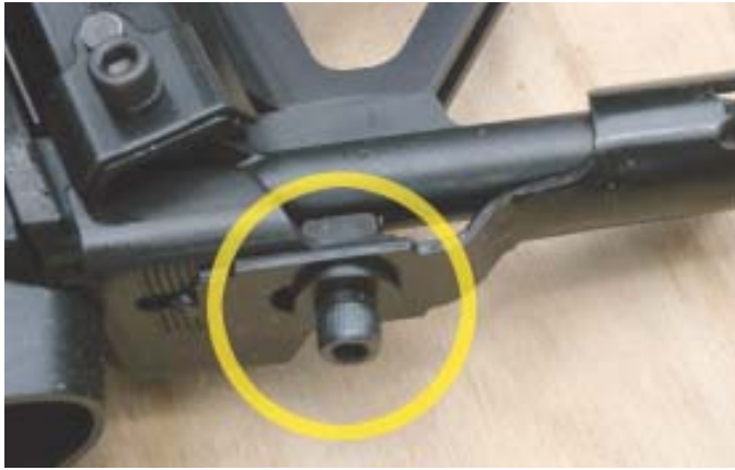
Figure 1. It takes an Allen key to adjust the depth of drive on this Duo-Fast gun. It works but is less convenient than a toolless mechanism.
