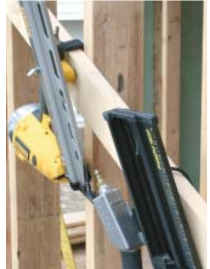
Figure 6. DeWalt's D51845 and Senco's 702XP were the only guns tested that have built-in rafter hooks — a must-have feature, according to the author (below). Guns without hooks tend to fall or get held in uncomfortable positions (left).
