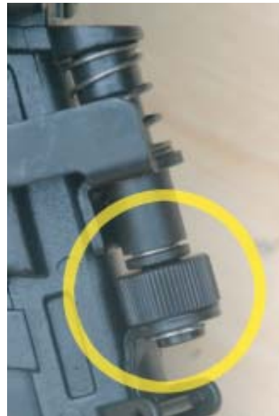
Figure 3. The thumb-wheel-activated depth control on this Porter-Cable nailer is typical of what you'll find on most newer framing guns.
