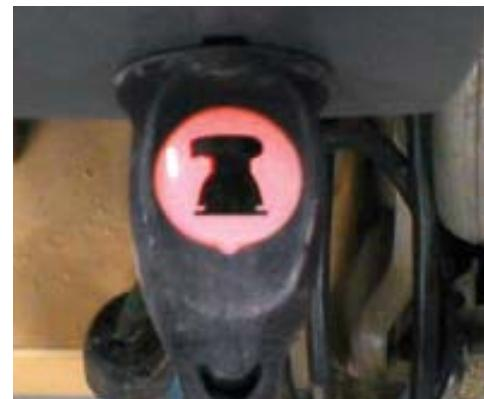
Included on all of the new Ridgid power tools, a light-up plug shows that you're plugged into a working receptacle. It also tells you what tool you're plugging in when you're dealing with a tangle of black cords.
