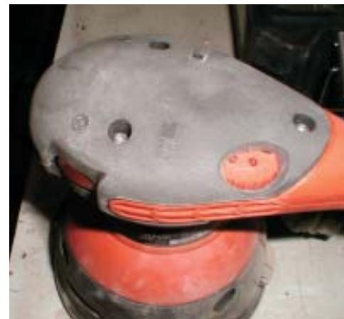
A little wheel on top of the housing adjusts speed from 7,000 to 12,000 rpm. The sander also has a pad brake to prevent the sanding disc from free spinning when you remove it from your work.
