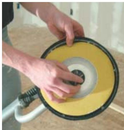
A large plastic nut secures the 9-inch sanding disc on Porter-Cable's drywall sander. The hook-and-loop disc is available in grits from 80 to 220 in packs of five. Replacement discs are packaged with a foam backing pad and sell for about \$22.
