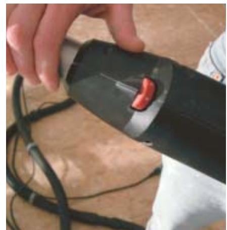
The red dial controls speed from 1,500 to 2,000 rpm. The variable-speed feature is handy while you're learning to use the tool, but once you get familiar with how it handles, there's no reason to go less than full power.
