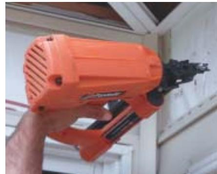
The IM200-S16 has a forked nosepiece, so one leg of the staple goes in the nail slot and the other goes above. The depth of drive is more consistent than that of a pneumatic stapler.
