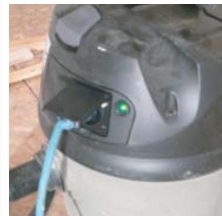
A green light tells you that a tool is connected and the vac is ready for dust collection. Once the tool is shut off, the vac continues running for a few seconds to clear the hose.
