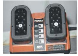
Because fast charging generates a lot of heat, the Ridgid two-bay charger uses a fan to cool the packs. Meshcovered holes in the pack allow air to reach the individual cells.
