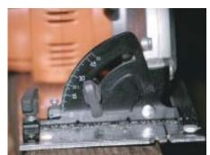
The cordless circular saw has a scale on the back of the blade guard that shows the depth of cut at a glance. The 6<sup>1</sup>/2-inch blade can cut through 2x framing material at a 50-degree bevel. White markings on a black background make depth and bevel settings easy to see.
