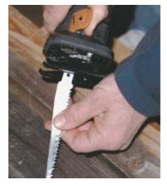
A small lever unlocks the blade clamp for easy changes. Blades can be installed upside down and even when the clamp is at the top of its stroke.
