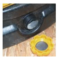
A threaded drain plug makes emptying a tank filled with water easy. A rubber gasket prevents leaks, and large knurls make the tool easy to grip, even with gloves on.
