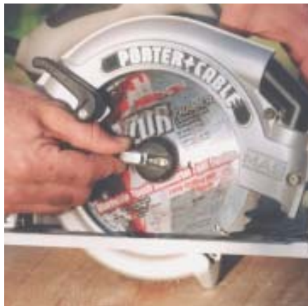
Figure 1. Porter-Cable's new toolless blade-changing system uses a knurled bolt and washer to keep the blade secure. A small lever (left) slides out to provide a grip and additional leverage. The design also puts the arbor lock on top of the saw (right) where it's easy to see and reach.
