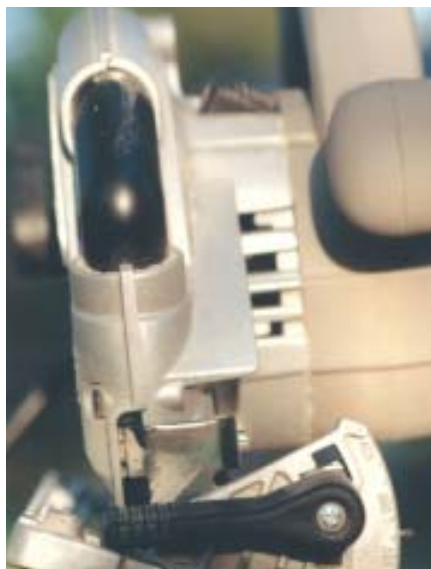
Figure 2. Unlike the removable dust nozzles on previous Porter-Cable sidewinders, the MAG series dust nozzle stores on the saw where it connects the front and back of the blade guard. It can be rotated about a half turn for directing dust away from your face or for use with a dust-collecting vacuum.
