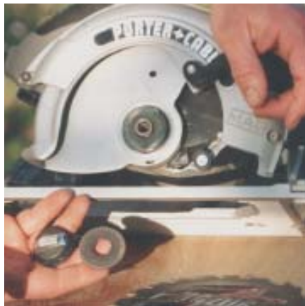
Figure 1. Porter-Cable's new toolless blade-changing system uses a knurled bolt and washer to keep the blade secure. A small lever (left) slides out to provide a grip and additional leverage. The design also puts the arbor lock on top of the saw (right) where it's easy to see and reach.
