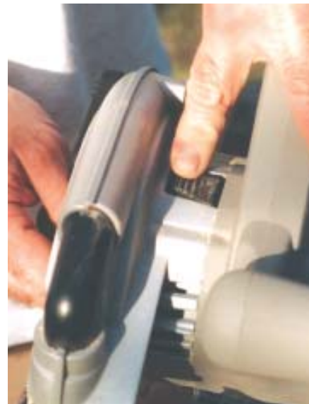
Figure 1. Porter-Cable's new toolless blade-changing system uses a knurled bolt and washer to keep the blade secure. A small lever (left) slides out to provide a grip and additional leverage. The design also puts the arbor lock on top of the saw (right) where it's easy to see and reach.
