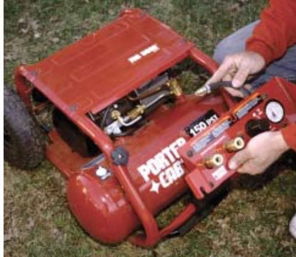
Figure 2. A removable control panel includes the air-pressure regulator and two push-in quick connects. The panel allows you to adjust air pressure from inside the house or up on a roof; the keyhole slot in the center of the panel allows you to hang it out of the way.
