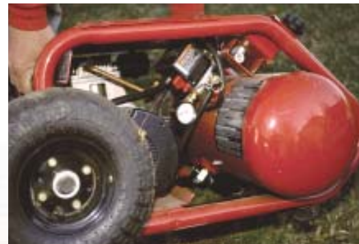
Figure 1. A steel roll cage protects all of the vulnerable components on the Job Boss compressor. Despite the added steel, the fittings and controls are still easy to get to. Pneumatic tires make it easy to move the compressor, even when climbing stairs.
