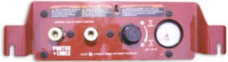
Figure 2. A removable control panel includes the air-pressure regulator and two push-in quick connects. The panel allows you to adjust air pressure from inside the house or up on a roof; the keyhole slot in the center of the panel allows you to hang it out of the way.
