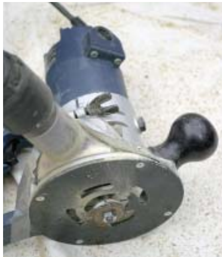
Figure 2. A bearing-over metric-sized bit is used to cut kerfs for the weatherstripping.
