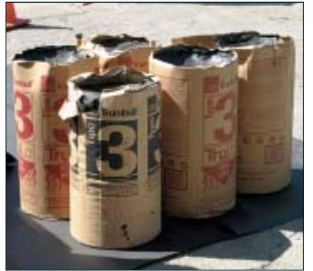
Figure 6. Different types of asphalt have different softening points. The type 3 material shown here softens at about 200°F but is applied at over 400°F.
