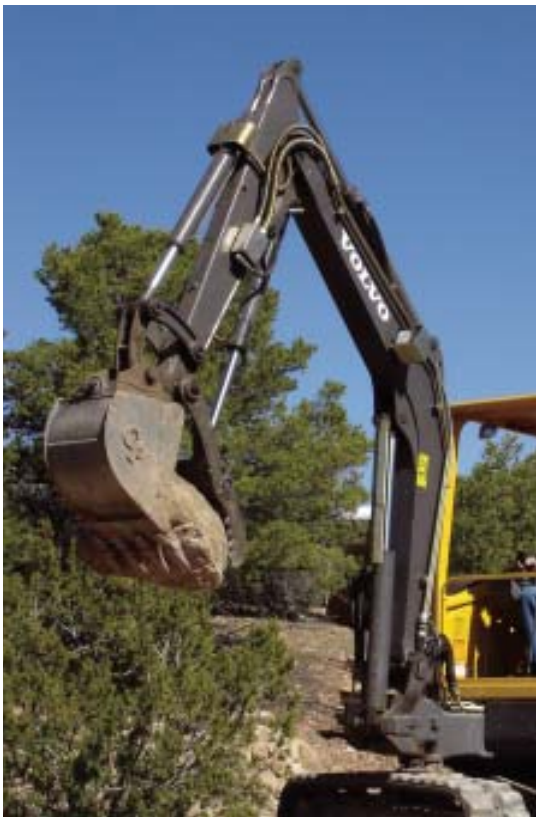
Figure 2. A hydraulic thumb makes it easy to pick up rocks and other large, odd-shaped objects that won't fit into the bucket. It's also a useful tool for demolition. When not in use, it folds against the boom.
