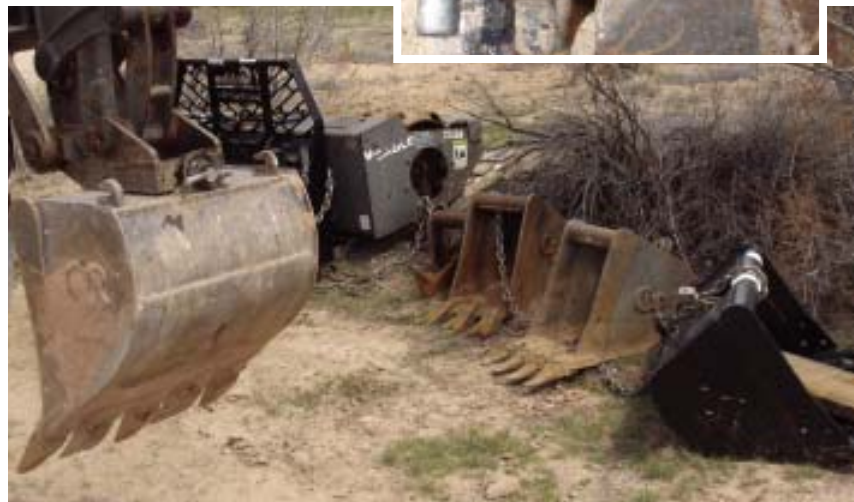
Figure 1. Quick couplers make swapping buckets and accessories much easier. With the hook end already on the bucket (top), the threaded pin is inserted and tightened (right). A whack with a hammer prevents vibration from loosening it, and a hitch pin keeps it from coming off if it should loosen.
