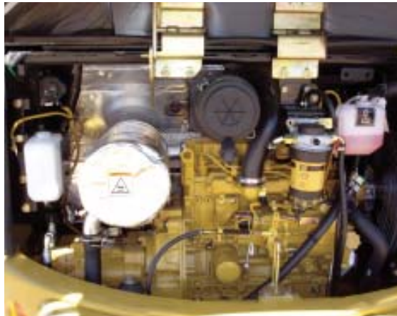
Figure 4. Although the newer machines have smaller engine compartments, manufacturers are doing a better job of keeping filters and other maintenance items easily accessible. This Caterpillar (top photos) has good filter accessibility despite its small engine-compartment door. With the Volvo (bottom photos), the oil filter is mounted lower in the engine compartment, so it's a little tougher to get to, but still reachable.
