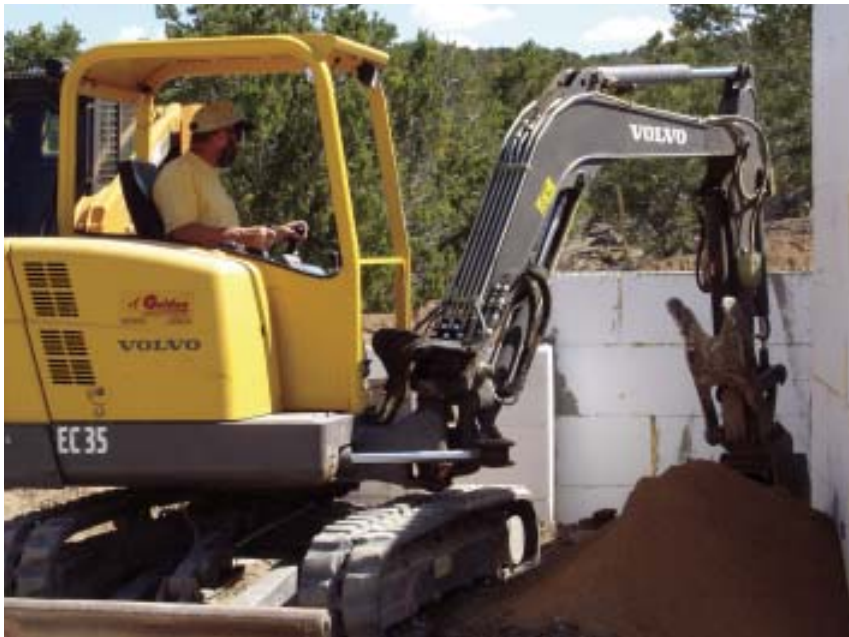
Figure 5. A major advantage of compact excavators is their ability to get close to foundations, fences, and obstructions. With the cab rotated and the boom angled to the left or right, excavators can dig in the offset position, which makes excavating for room additions and trenching next to foundations easier.
