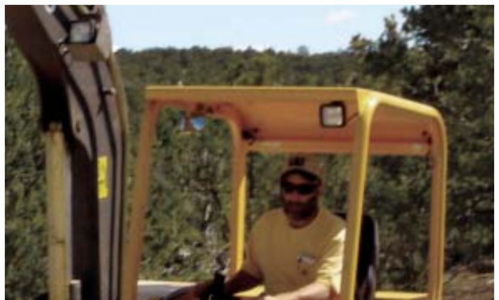
Figure 3. A light kit is a worthwhile accessory, especially when you're struggling to finish a job. The most useful kits have lights for the front and back of the cab for crawling in either direction, and on the boom to see inside a trench or hole.
