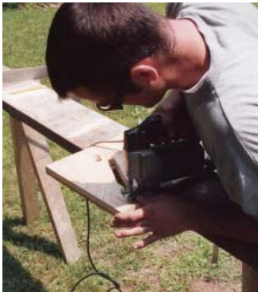
Figure 2. Because the site-built jig will guide the router, it's important to cut the template carefully. Here, a carpenter makes the first plunge cuts with a circular saw (far left) and then finishes up with a jigsaw (left).
