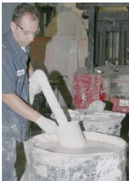
A technician pumps paint out of a barrel through filters (left) and into a 500-gallon vat (above). Then a giant mixer blends the paint with pigment and additives.
