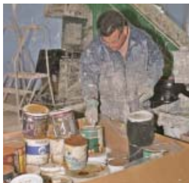
AEI's crew sorts paint by color and quality (above) before draining it into barrels (right).
