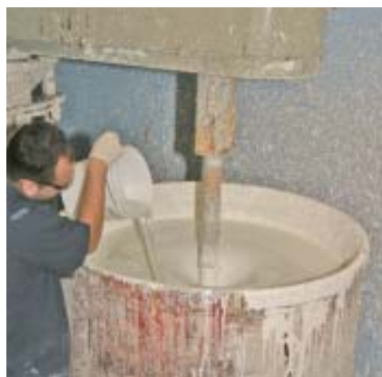
A technician pumps paint out of a barrel through filters (left) and into a 500-gallon vat (above). Then a giant mixer blends the paint with pigment and additives.
