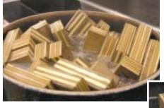
In a two-cycle boil test, samples of plywood made with a soy-based adhesive are submerged in boiling water for four hours and dried for 20 hours, then boiled again for four hours and dried for another 20. Even after such rigorous treatment, the samples do not delaminate.
