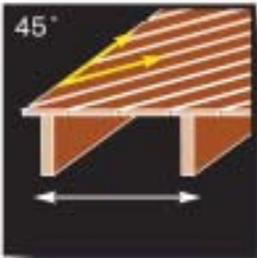
At a 45° angle, maximum joist spanning is 4" less than above chart.
