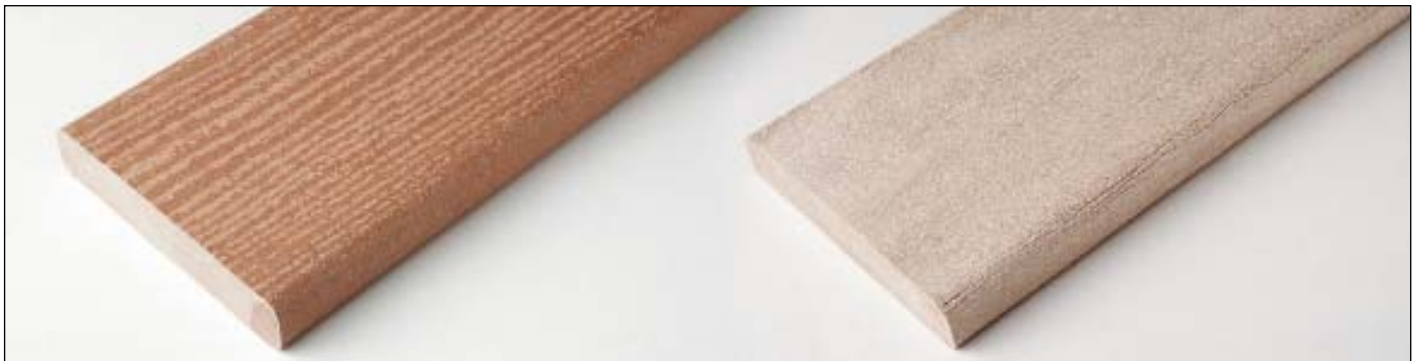
FIGURE 4. In the long run, composite decking will likely weather the sun, rain, and ice much better than pressure-treated lumber. Ultraviolet light will fade the top surface of composite materials (shown new at left), but the material remains serviceable and does not usually continue to degrade after initial weathering.
