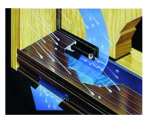
ting sweep requires extra force to close the door, and the constant opening and closing eventually reduces the arrangement's effectiveness. Hydrosill's two-tiered sill channels water back outside — plus a Q-LON foam gasket provides a tight seal without the typical drag and wear problems. The Hydrosill comes in sizes suitable for standard entry doors, swinging patio doors, and entry systems with sidelights. A 3-foot version for a 2x4 wall costs about \$26.
