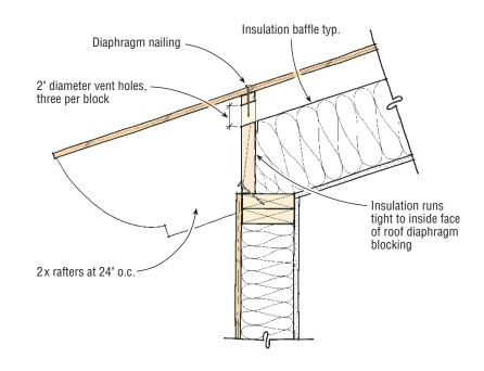
inch, with a one-third increase allowed for dynamic (seismic or wind) loading. If the 2-by rafters are spaced 24 inches on-center, the blocks are 22<sup>1</sup>/2 inches long. Assume that for venting you
