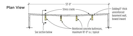
Reinforced concrete buttresses connected to the existing foundation wall and slab floor with epoxied rebar dowels should prevent further movement in this bowed basement wall.
