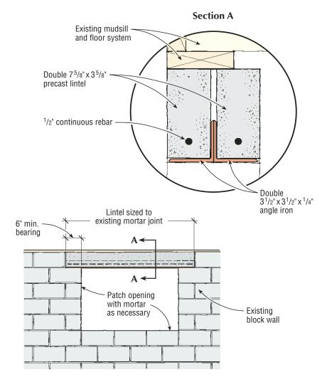
When cutting an opening in an existing block wall, try to align it with existing mortar joints, and size the new lintel so that it is supported by at least 6 inches of block on either side. Though structurally unnecessary, a pair of angle irons provides extra support that helps eliminate minor cracking in doubled-up precast lintels (Section A).
