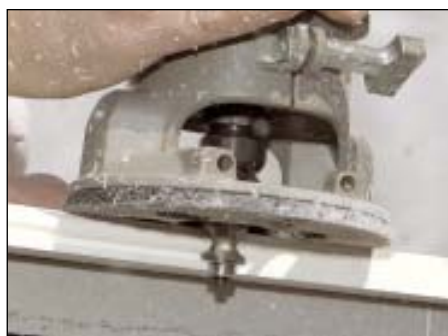
FIGURE 1: PVC trim stock cuts and routs much like wood. The dust tends to have a static cling, but it's not as fine or as abrasive as fiber-cement dust. PVC trim also won't dull blades any faster than wood.
