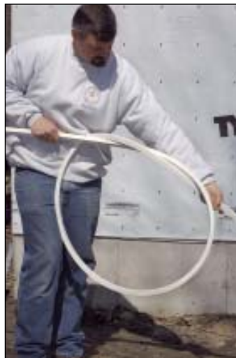
FIGURE 4: PVC trim stock is much more flexible than wood of comparable dimension. It will sag on a table saw, so two people are needed to rip it. To demonstrate the material's flexibility, the author ties a 1-inch-wide strip into a pretzel.
