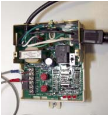
Figure 9. An the installer inserts a heat sensor into a flat-plate collector (above left); this sensor and another one on the storage tank connect to an electronic controller (left) that activates the pump (top center in photo above) whenever the collector is 5°F hotter than the tank.
