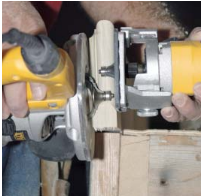
Figure 1. For the look of a traditional stool, the author uses full 1-inch-thick stock profiled with a router. He shapes the bottom edge with a cove-and-bead bit and the top edge with a 5/16 -inch roundover bit. At right, the finished edge profile with the router and trimmer held in place.
