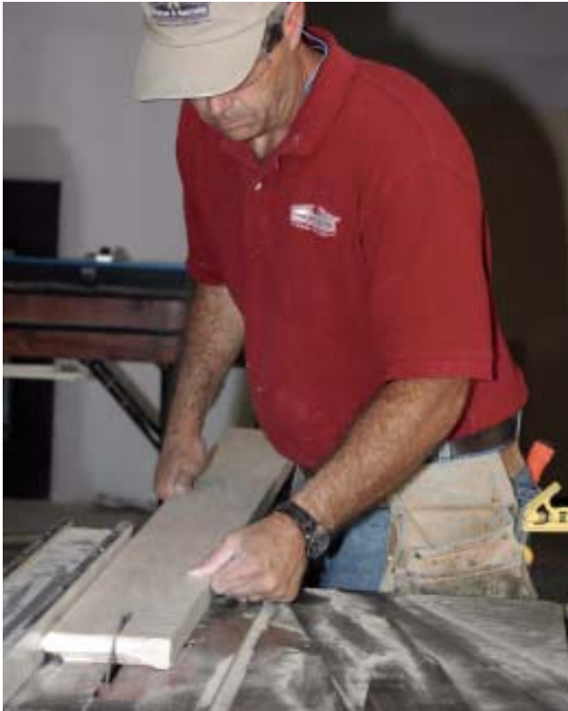
Figure 2. It helps to have the right tools: The author uses a table saw to cut the ears on the stool (left) and a jointer to taper the extensions so they match the plane of the drywall next to the window (below). A Kreg machine makes quick work of boring pocket holes (bottom).
