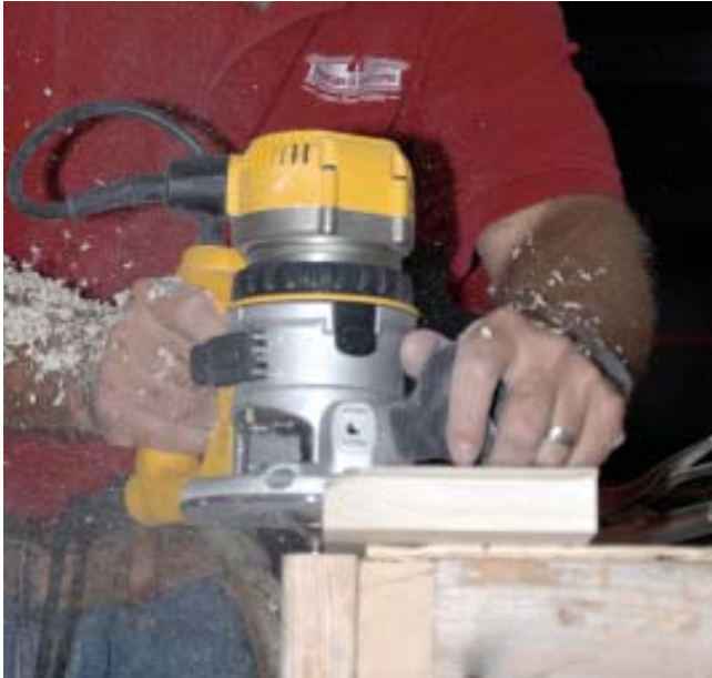
Figure 1. For the look of a traditional stool, the author uses full 1-inch-thick stock profiled with a router. He shapes the bottom edge with a cove-and-bead bit and the top edge with a 5/16 -inch roundover bit. At right, the finished edge profile with the router and trimmer held in place.
