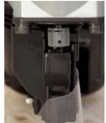
Figure 3. Depth-of-drive mechanisms are standard on every framing nailer. The button on the tip of the Bostitch (above left) makes for quick and intuitive depth changes. Dial mechanisms like the one on the Hitachi (above) are fairly common and work quite well. The old-fashioned depth mechanism on the Porter-Cable gun (left), similar to that on the Paslode, requires the use of an Allen key.
