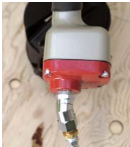
Figure 5. Max's gun has a swivel air fitting that prevents kinking and reduces wear on the hose.
