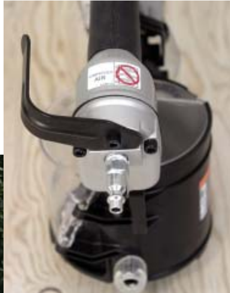
Figure 4. Makita's gun (right) comes with a built-in hook that allows you to hang up the tool. This carpenter (below) frees his hands by hanging the tool from his belt.
