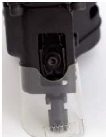
Figure 3. Depth-of-drive mechanisms are standard on every framing nailer. The button on the tip of the Bostitch (above left) makes for quick and intuitive depth changes. Dial mechanisms like the one on the Hitachi (above) are fairly common and work quite well. The old-fashioned depth mechanism on the Porter-Cable gun (left), similar to that on the Paslode, requires the use of an Allen key.
