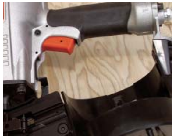
Figure 6. The Paslode's smooth, over-size trigger is more comfortable to use than the triggers on the other guns.
